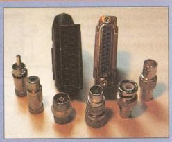
Don't get confused by the different types of video connector, especially if you're new to video. The ones pictured here are (clockwise, from right) BNC socket, BNC plug, RF plug, RF socket, Phono socket, Phono plug, SCART connector, 23pin D connector (Amiga RGB port).
